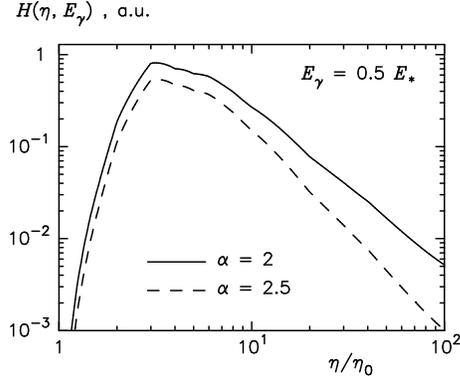
Figure 13: Function  $H(\eta, E_\gamma)$  at fixed energy of  $\gamma$ -rays,  $E_\gamma = 1/2 E_*$ , calculated for a power-law distribution of protons  $f_p(E_p) \propto E_p^{-\alpha}$  with  $\alpha = 2$  and  $2.5$ .
