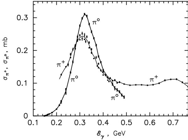
Figure 9: The total cross-sections of production of  $\pi^+$  and  $\pi^0$ -mesons as a function of energy of incident gamma-ray in the rest frame of proton. The experimental points are taken from the site <http://wwwppds.ihep.su:8001>.
