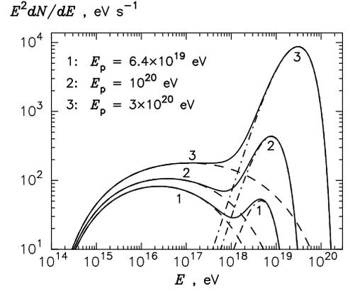
Figure 10: Energy distributions of electrons and positrons ( $N_e = N_+ + N_-$ ) produced at interactions of protons with 2.7 K CMBR. Dashed lines and dot-dashed lines correspond to the pair production and photomeson processes, respectively. Solid lines show the sums of two contributions. The curves correspond to three energies of protons:  $6.4 \times 10^{19}$  eV,  $10^{20}$  eV and  $3 \times 10^{20}$  eV.
