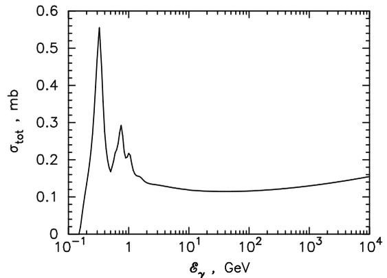
Figure 1: The total cross-section of the inelastic  $\gamma$ - $p$  interactions as a function of energy of gamma-ray in the proton rest frame. The calculations have been performed using the routine of the code SOPHIA [11].
